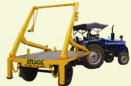
Container Lifting Device
