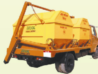
DP System (3.5 m 3 -Twin Container)
