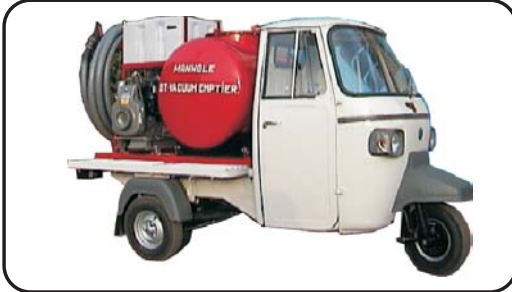
Rikshaw Mounted Manhole Vacuum Emptier
