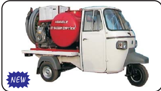
Rikshaw Mounted Manhole Vacuum Emptier
